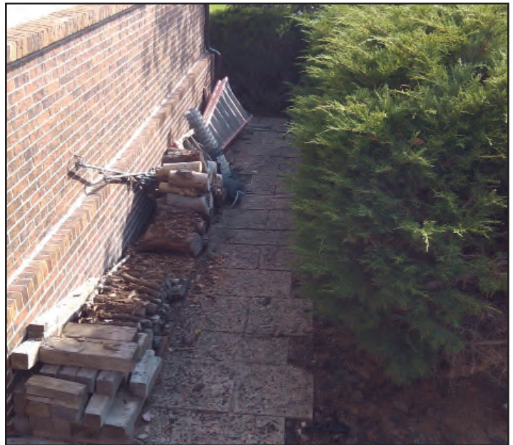
This firewood pile is beside a brick wall, but it also is bordered by a large juniper. If both the firewood pile and juniper are burning, they could produce enough heat to impact the stucco wall and eaves. The pile below is better located because it is away from the home and at a similar level. Photos by South Metro Fire Rescue.
