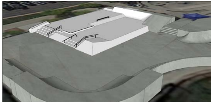
The new design will be more durable and will incorporate grind rails, banks, steps, ledges and vertical drops that will flow into the existing quarter pipes.
